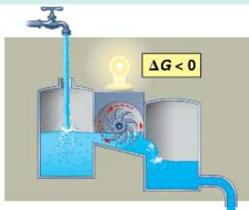
(b) An open hydroelectric system
