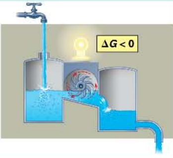
(b) An open hydroelectric system
